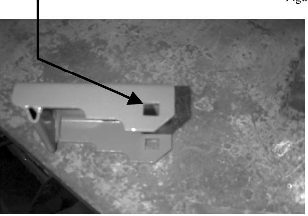
Square Holes in the Side of the Uplock Jaw (File Paint off of the Inside surface of the Holes)
