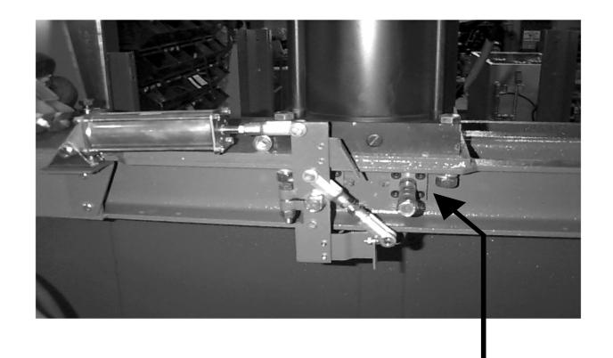
Right-Hand Side Lock Shaft Bearing
